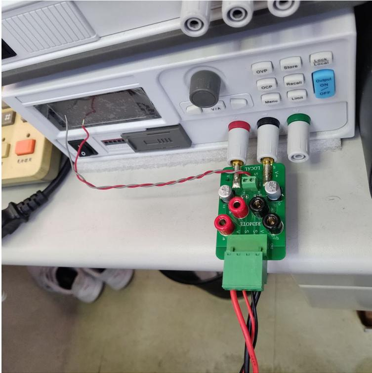
Figure 8: The PWR-OPT05 remote sense board connected to the P9610 power supply with the remote sense line along with DC voltage (larger gauge) and sense lines going out to power the DUT and sense it's input voltage.
