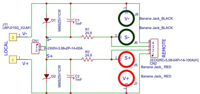
Figure 7: Sample remote sense filter along with the PWR-OPT05 schematic.
