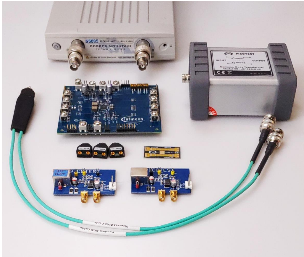
Fig. 2 - Picotest J2102B ground isolator, calibration substrate, P2102A probe with cables, P2102A probe tips, Infineon PS5401 Eval DUT, Picotest LM20143 DUTs, and Copper Mountain Technologies Compact S5085 VNA
