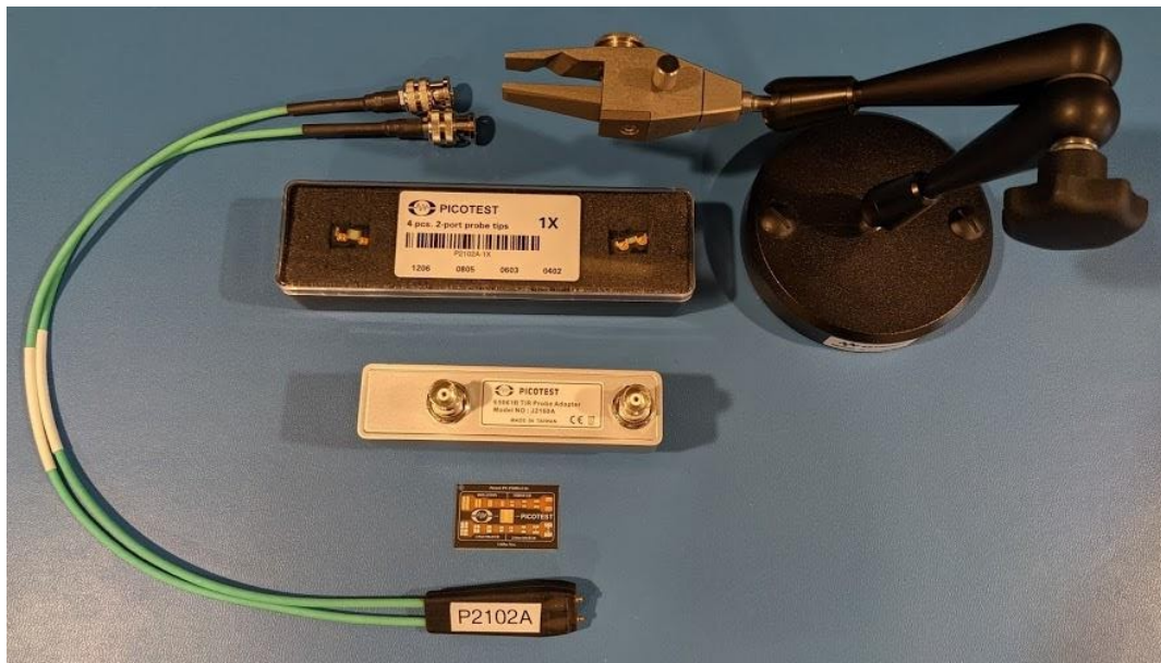
Fig. 3 - Picotest P2102A probe, P2102A probe tips, J2160A, calibration substrate, and probe holder for measurement (for use with the low frequency-RF(T/R) BNC-conductor ports).
