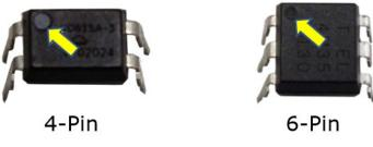
Fig. 2 - Depiction of 4-pin and 6-pin Optocoupler Packages.
