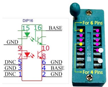
Fig. 3 - J2200A Socket Connection Diagram.
