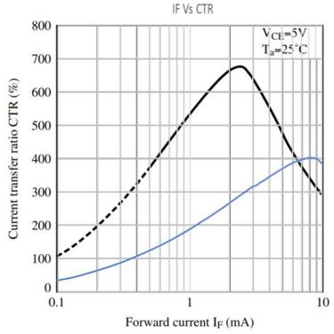
Figure 8 - PC817X Overlay of Measured CTR (blue) and Datasheet CTR (black).
