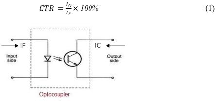
Fig. 1 - Typical Optocoupler Diagram.
