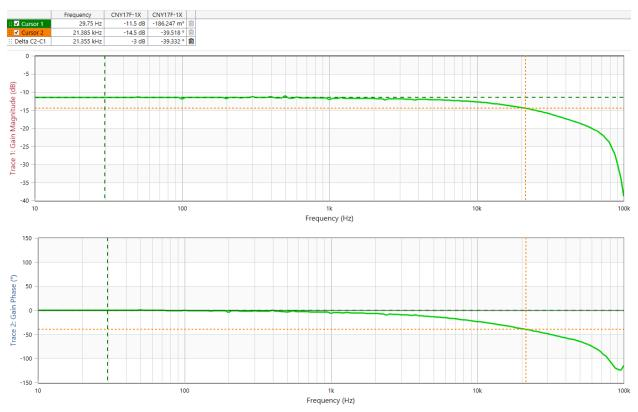
Fig. 11 - CNY17F-1 Gain and Phase Measurement Result with J2200A and Bode 100.
