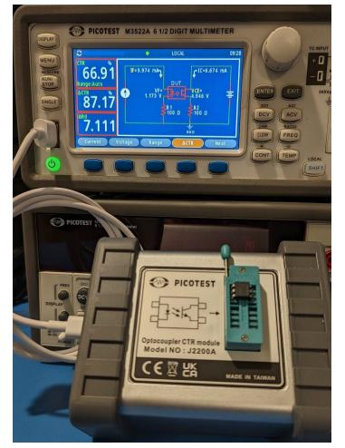
Fig. 5 - LITE-ON CNY17F-1 CTR Measurement Result on M3522A DMM.
