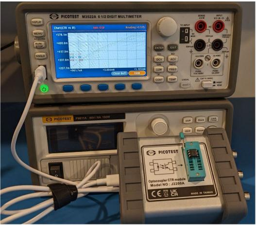
Figure 7 - CTR vs. IF Result of CNY17F-1 Optocoupler.
