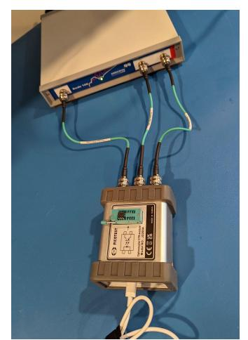
Fig. 10 - Measurement Setup with J2200A and Bode 100.
