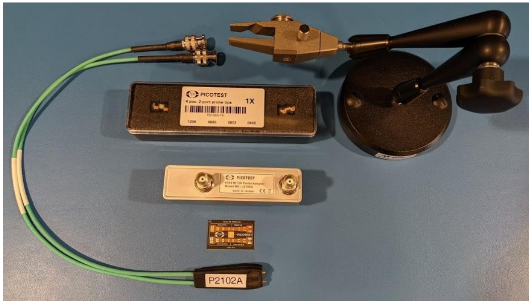
Fig. 3 - Picotest P2102A probe, P2102A probe tips, J2160A, calibration substrate, and probe holder for measurement (for use with the low frequency-RF(T/R) BNC-connector ports).
