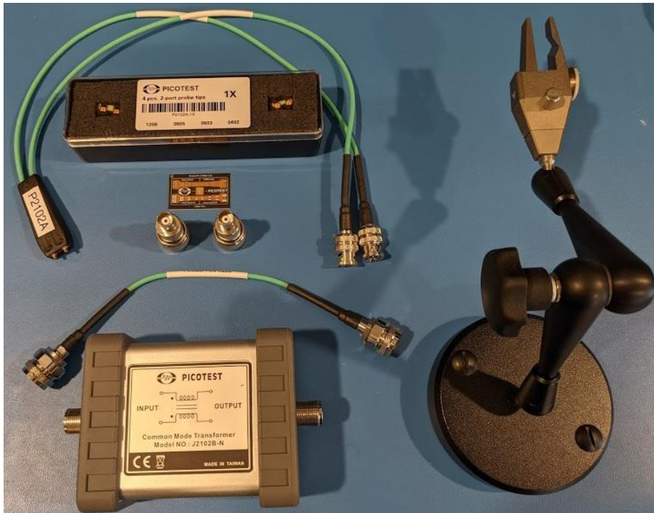
Fig. 2 - Picotest P2102A probe, P2102A probe tips, Picotest PDN Cable, J2102B ground isolator, adapters, calibration substrate, and probe holder for measurement (for use with the Port 1-Port-2, N-connector S-parameter ports).
