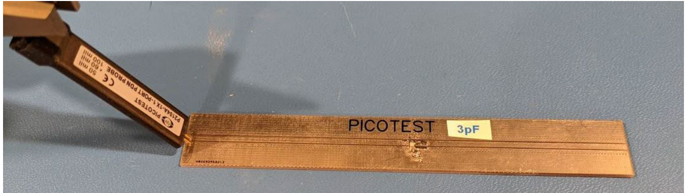
Fig. 12 - TDR Measurement Setup for a 3pF Capacitor Test PCB with the P2104A Probe and J2154A TDR.
