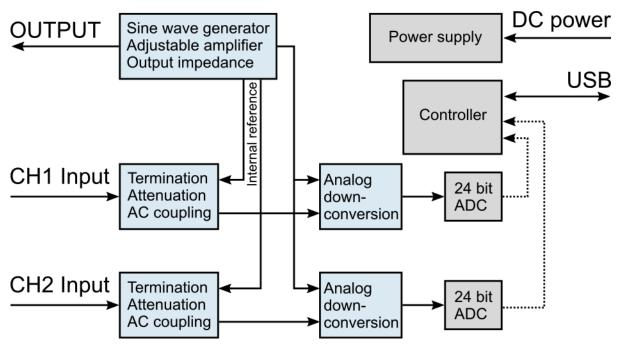
Figure 5-3: Bode 100 block diagram
