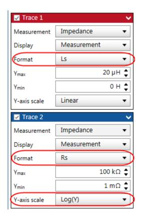
To get a better view on the Ls and Rs it is recommended to **switch to two diagrams**. To do so follow the instructions described in 9.3.1 Configure the diagrams on page 101.
