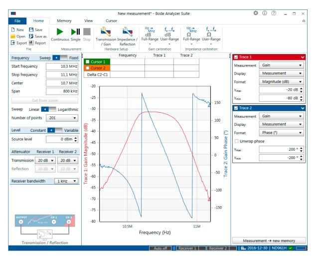
Figure 9-15: Phase-wrap effect caused by the fact that phase can only be measured between -180° and +180°
