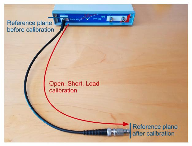
Figure 8-4: Shifting the reference plane by performing Open, Short and Load Calibration
