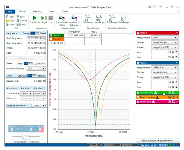
Figure 9-12: Using the memories to compare different measurements
