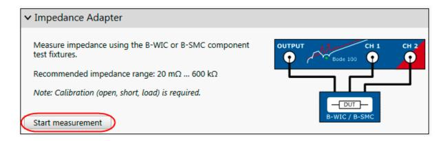
Before you can start a measurement you have to perform a **Full range calibration**. To do so please follow the steps described in Impedance Adapter Calibration on page 82.
