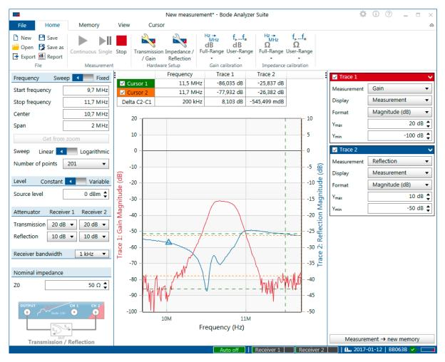
Figure 7-2: S-Parameter measurement of a 10.7 MHz IF filter
