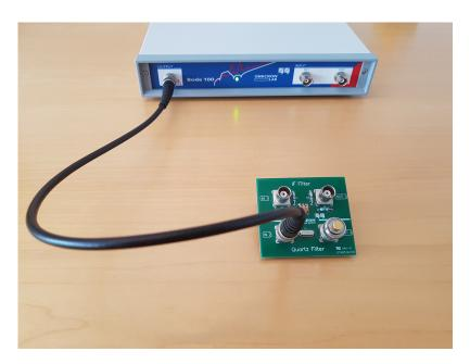
Figure 7-6: Connecting the test object Quartz Filter to Bode 100
