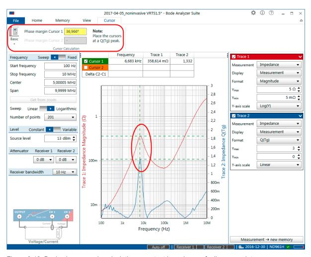
Figure 9-13: Basic phase margin calculation on output impedance of a linear regulator. The result shows a phase margin of nearly 37° (yellow) after placing cursor 1 to the peak in Q(Tg).
