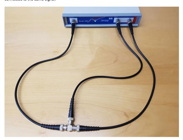
Figure 8-2: Thru calibration setup for gain/phase measurement with BNC cables.
