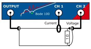
Use a 1  $\Omega$  resistor for Thru calibration. 1  $\Omega$  results in 1 V/A. Thru calibration can e.g. remove the gain and phase error introduced by the probes. However, it does not correct for systematic measurement errors in the measurement setup such as a voltage drop on the current probe or the current flowing through the voltage probe. These errors cannot be removed by one calibration measurement. In such a case you can use Open/Short/Load calibration to reduce these errors.
