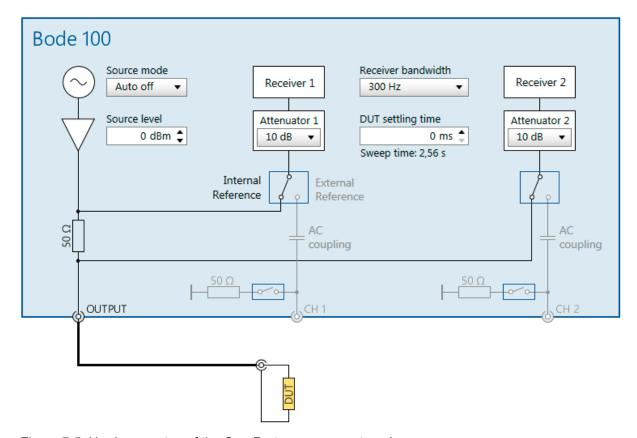
Figure 7-5: Hardware setup of the One-Port measurement mode.
