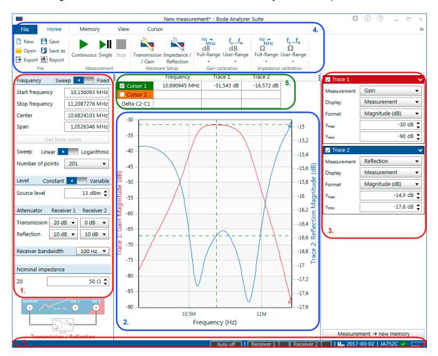
Figure 6-2: Bode Analyzer Suite Main window.
