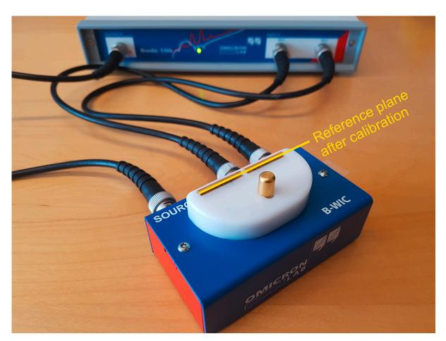
Figure 8-6: Calibrating the B-WIC impedance test fixture by performing Open, Short and Load Calibration
