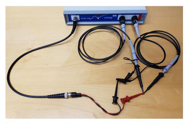
Figure 8-3: Thru calibration setup for gain/phase measurement using scope probes.
