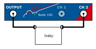
Thru calibration can e.g. remove the gain and phase error introduced by the connection cables including a coaxial common mode transformer that is generally used in this measurement to suppress the cable-braid error.
