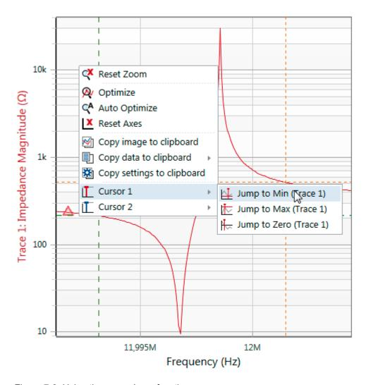
Figure 7-9: Using the cursor jump functions
