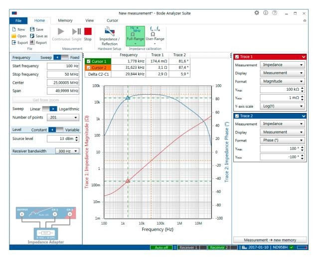
Figure 7-13: Impedance measurement of an Inductor
