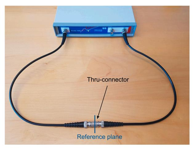
Figure 8-1: Gain, respectively Thru calibration setup in a transmission measurement.
