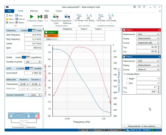
Figure 9-16: Unwrapped phase result shows the total phase shift of the IF filter DUT
