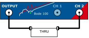
Thru calibration can e.g. remove the gain and phase error introduced by the connection cables.
