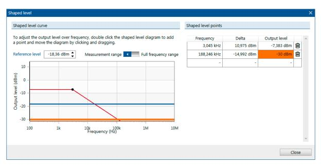
Figure 9-2: Output level limited to the minimum output level of the device
