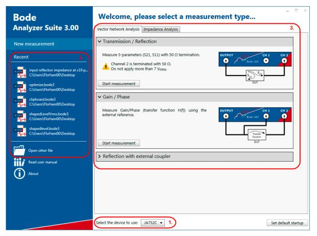
Figure 6-1: Bode Analyzer Suite Start screen.
