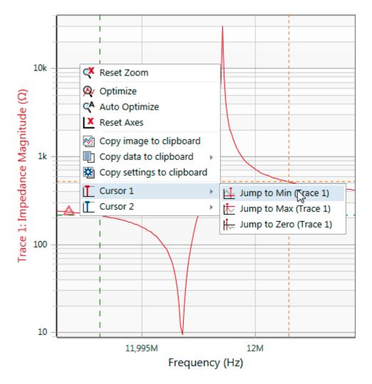
Figure 7-9: Using the cursor jump functions
