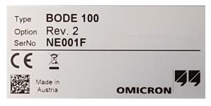
Your identification plate might look slightly different. The important information is visible in the Option field. If Option is Rev. 2, you are using a Bode 100 R2. If Option is empty, you are using a Bode 100 R1.
