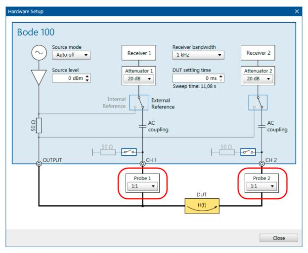
Figure 9-15: Probe configuration in the hardware setup dialog
