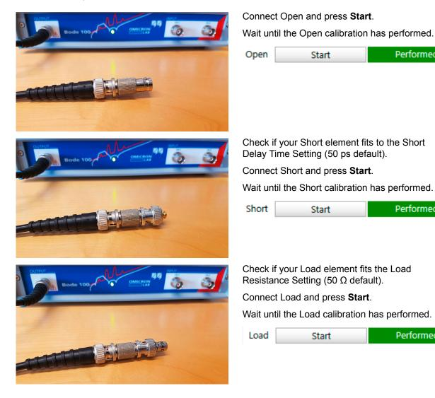
٢ Hint: The load delivered with the Bode 100 is marked with its exact impedance. You can improve the calibration accuracy by entering this value in the Advanced Settings area. The Short Delay Time in the Advanced Settings area has been chosen to match the Short elements delivered with Bode 100. If your short is marked with Rosenberger you can set the Short Delay Time to 40 ps, if it is marked with Radiall to 60 ps.
