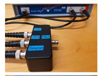
Connect Open and press **Start** . Wait until the Open calibration has performed.
