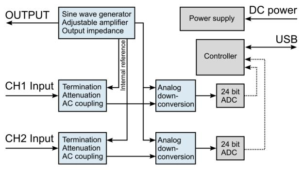
Figure 5-3: Bode 100 block diagram
