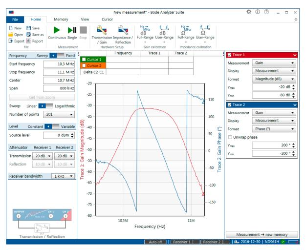
Figure 9-16: Phase-wrap effect caused by the fact that phase can only be measured between -180° and +180°  $\,$
