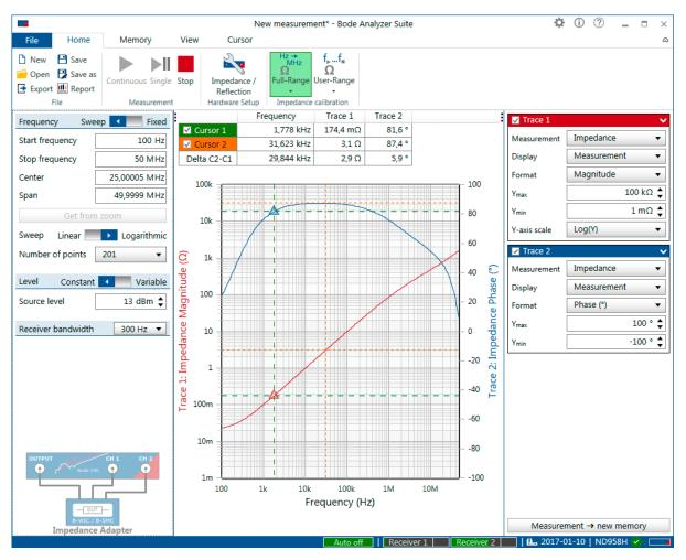
Figure 7-13: Impedance measurement of an Inductor
