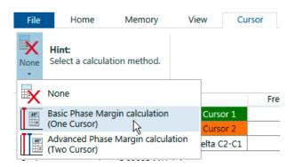
As a next step, follow the instruction in the GUI and place Cursor 1 to the peak in the Q(Tg) result. The phase margin calculation method shows the phase margin result in the cursor ribbon as shown in the following figure:
