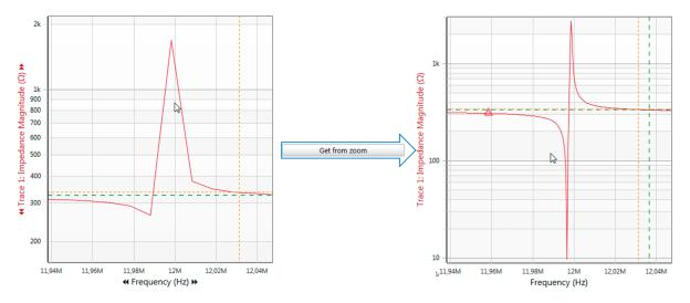
Figure 7-8: Optimizing the frequency resolution with Get from zoom
