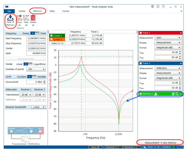
Figure 9-11: Using of memory curves to see changes in the measurement and to compare different curves
