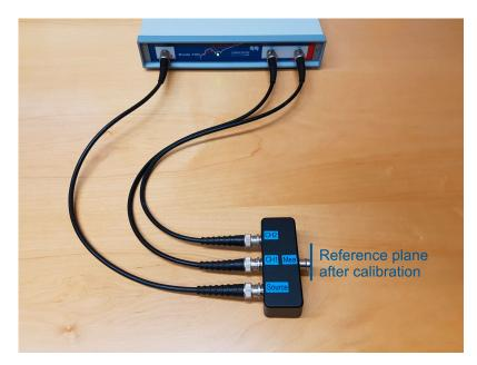
Figure 8-5: Removing a coupler / bridge by performing Open, Short and Load Calibration
