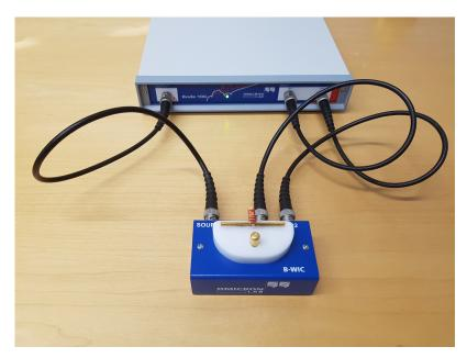
Figure 7-12: Connecting the *B-WIC* to *Bode 100*
