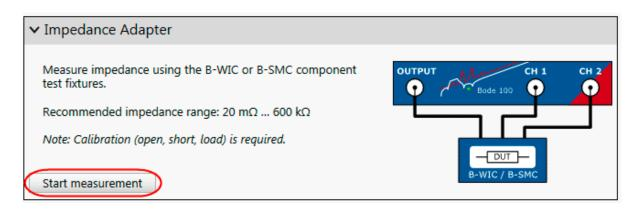
Before you can start a measurement you have to perform a **Full range calibration**. To do so please follow the steps described in Impedance Adapter Calibration on page 82.
