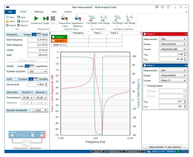
Figure 9-3: Two measurement traces in one diagram
