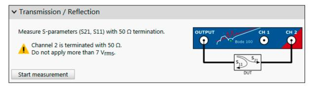
The Transmission / Reflection measurement mode allows to measure both, Transmission (Gain) and Reflection (Impedance). It is possible to select e.g. a Gain measurement in Trace 1 and an Impedance measurement in Trace 2. *Bode 100* will then sequentially measure Gain and Impedance.
