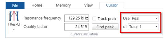
In this example we want to calculate the resonance frequency and Q-factor based on the Real part of the values in Trace 1. As an alternative also the Magnitude can be used. If multiple traces contain values or if a memory is linked to the cursor table, then the calculation can also be applied to these curves.
