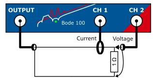
Use a 1  $\Omega$  resistor for Thru calibration. 1  $\Omega$  results in 1 V/A. Thru calibration can e.g. remove the gain and phase error introduced by the probes. However, it does not correct for systematic measurement errors in the measurement setup such as a voltage drop on the current probe or the current flowing through the voltage probe. These errors cannot be removed by one calibration measurement. In such a case you can use Open/Short/Load calibration to reduce these errors.
