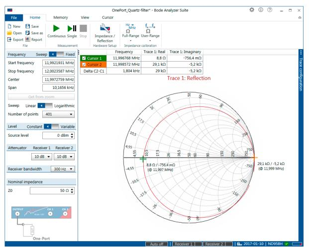
Figure 7-11: Smith chart of the 12 MHz Quartz Filter
