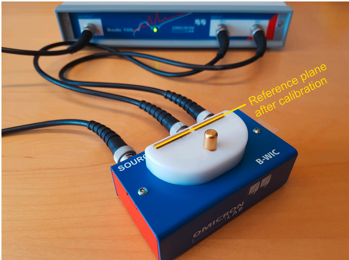
Figure 9-6: Calibrating the B-WIC impedance test fixture by performing Open, Short and Load Calibration
