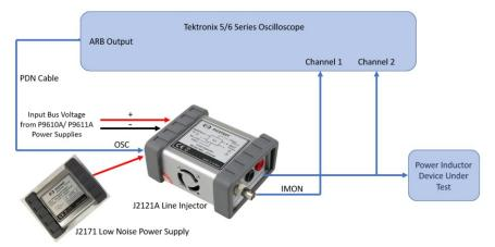
DC biased inductor measurement setup using a Tek MSO and J2121A line injector. The  $\pm$ 12V supply to the line injector is fed from (included) J2171A power supply. The DUT inductor is connected in 2-port shunt-through configuration. The J2121A current monitor ( $\pm$ 10) output is connected to CH1 of the oscilloscope. The oscilloscope ARB (arbitrary waveform generator) oscillator is connected to modulation input of the J2121A.
