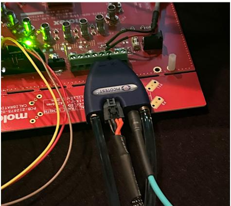
The compact head on the P2124A probe eliminates interconnect inductance by bringing the line injector electronics into the probe head.
