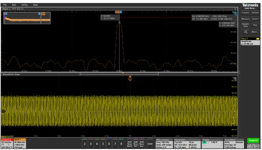
The P2124A modulates the bus voltage into a 0.6 Ohm Load with 5.5Amp DC Bias and 40MHz operation.
