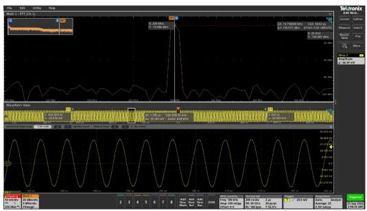
While the response is attenuated, increasing the input modulation source level achieves modulation up to 250MHz.
