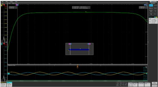
P2124A Probe 3dB Bandwidth 29.27Hz - 38.887MHz 0.6 Ohm Load with 5.5Amp DC Bias.
