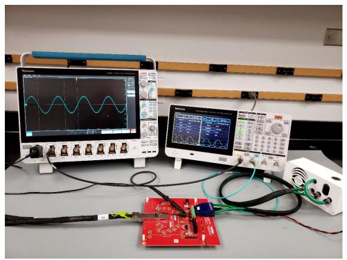
Sample PSNR Test Setup using the Picotest P2124A and the Molex Transceiver board.
