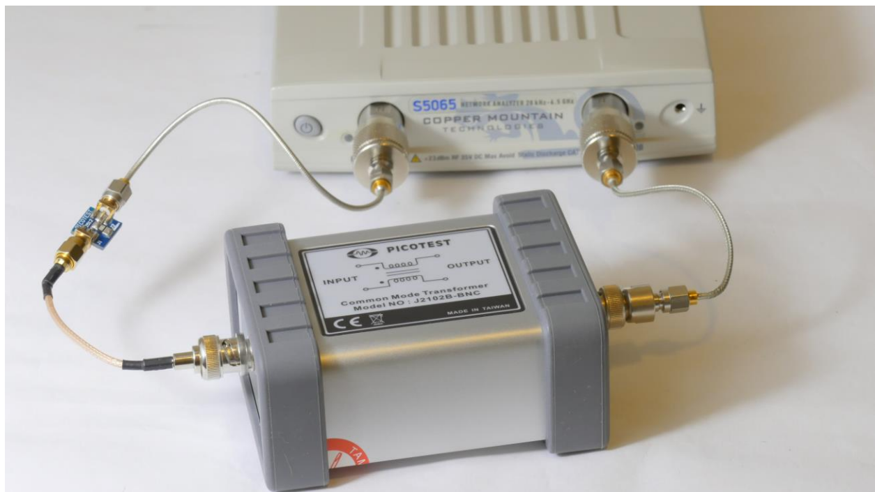
The J2102B common mode transformer is used to break the instrumentation ground loop in this 2-port shunt-through impedance test setup of a decoupling capacitor using the Copper Mountain S5065 VNA.
