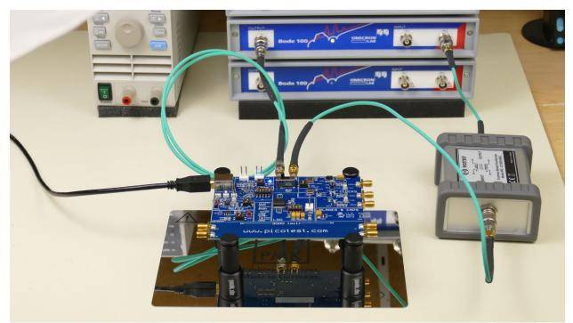
The Picotest PDN Cables and the J2102B Common Mode Transformer combine to enable the 2-port
