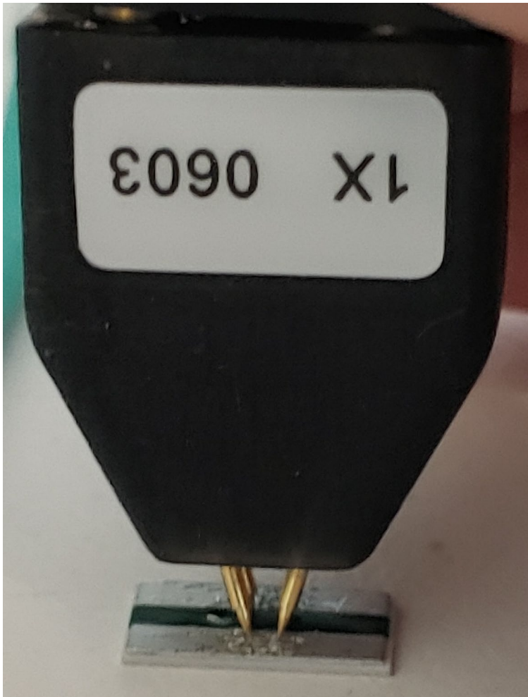
Figure 6: A 2-port measurement using the P2102A probe. Pressure is needed to seat the four pins firmly in place. The probe head should match or be larger than the capacitor you are measuring across. Two pins go on each side of the capacitor.
