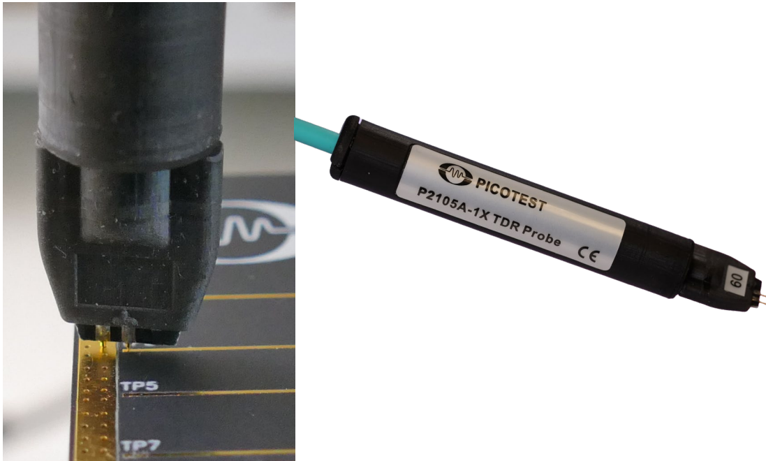
Figure 4: P2105A TDR probe. The P2105A 1-port probe comes in fixed pitch widths of 31, 40, 50, 60, 70, 100mils and GSG SMA. Custom pitches are also available.
