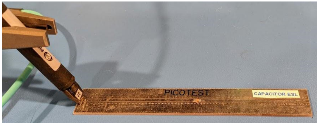
Fig. 18 - TDR Measurement Setup of Series Capacitor ESL with the P2105A Probe.
