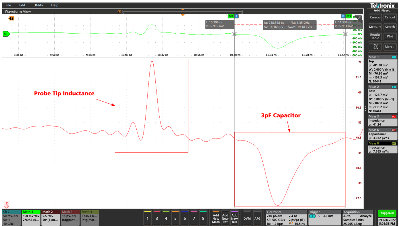
Fig. 14 - TDR Measurement Result of the 3pF Capacitor with the P2104A Probe and J2154A TDR.
