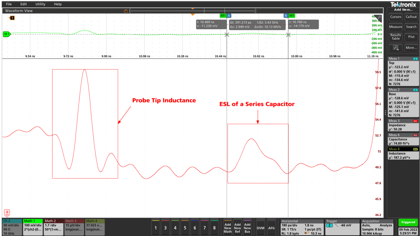
Fig. 19 - TDR Measurement Result of Series Capacitor ESL with the P2015A Probe.
