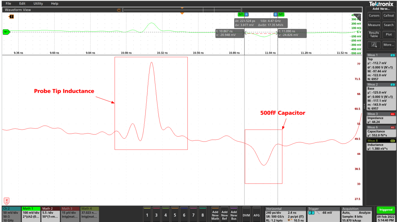
Fig. 16 - TDR Measurement Result of a 500fF Capacitor with the P2104A Probe and J2154A TDR.
