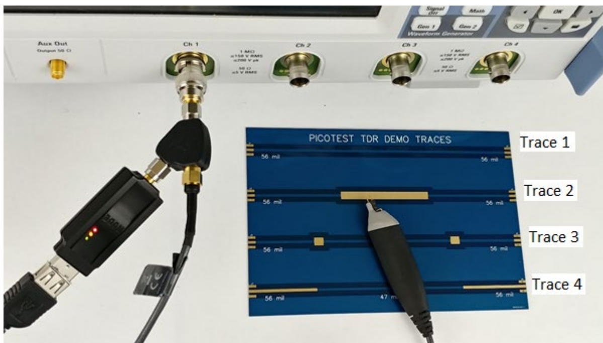
Figure 2: Picotest TDR demo board.
