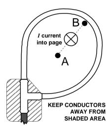
The sensitivity of the CWT to currents that do not pass through the coil is very small, provided that such currents are no greater than the CWT's rating or such currents are relatively distant from the coil. In the vicinity of a multi-turn inductor the 'H' field is far stronger than from a single conductor carrying the same current, and such positions should be avoided.
