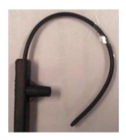
When clipping or unclipping the coil, hold the ferrule as shown
