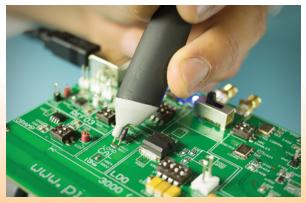
1 Port PDN Transmission Line Probe
