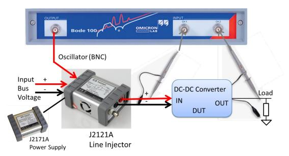
Figure 16: J2121A Line Injector Connections for PSRR measurements.
