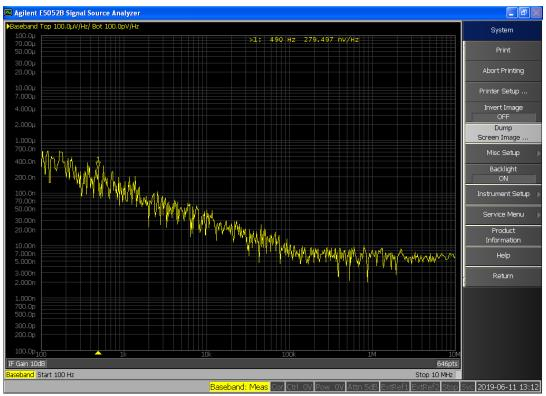
Figure 57: J2161A Typical Noise Density plot.
