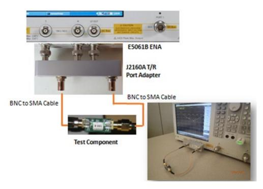
Figure 59: Measuring Components Using the Keysight E5061B GP Ports (Low Frequency).
