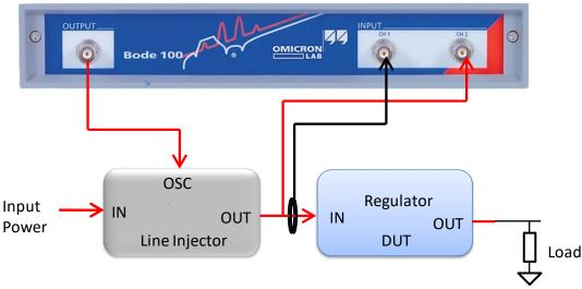
Figure 13: Line Injector Connections for input impedance measurements.
