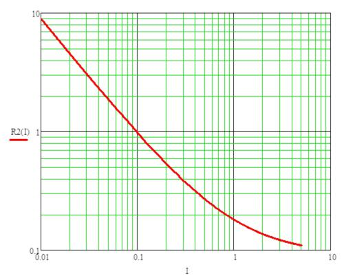
Figure 15: Line Injector output resistance.
