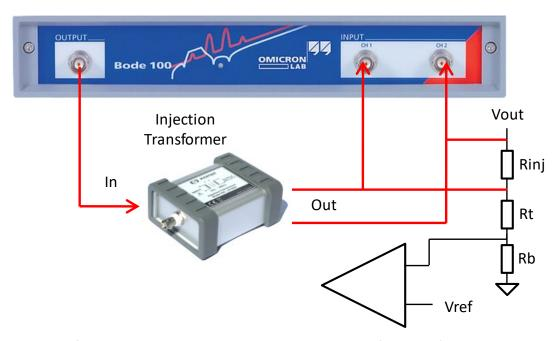
Figure 1: Sample setup for the injection transformer (J2100A or J2101A) used to perform stability measurements.
