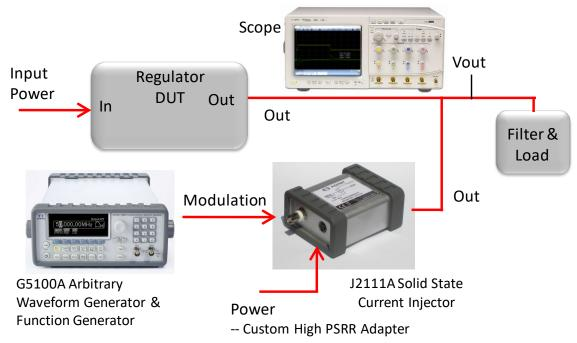
Figure 3: Sample setup for the Solid-State Current Injector (J2111B) used to perform a non-invasive load transient measurement.
