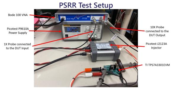
Figure 20: Line Injector Connections for PSRR measurements.
