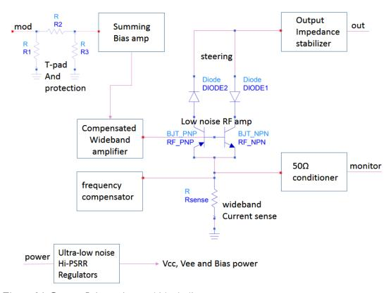
Figure 26: Current Injector internal block diagram.
