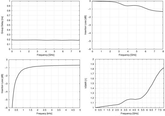
Figure 25: Electrical performance characteristics of the P2130A DC blocker.
