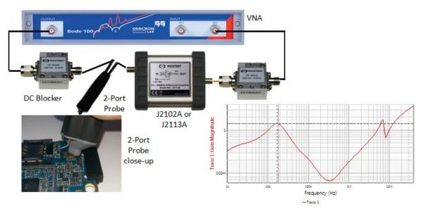
Figure 44: Measuring the in-circuit output impedance using the Picotest P2101A 2-Port Transmission Line Probe. The J2102A has been replaced by the J2102B.
