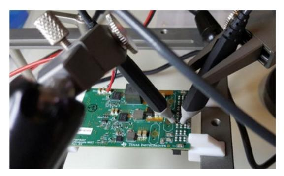
Figure 46: Setup image of the in-circuit 2-port impedance measurement using two 1-Port PDN Probes.
