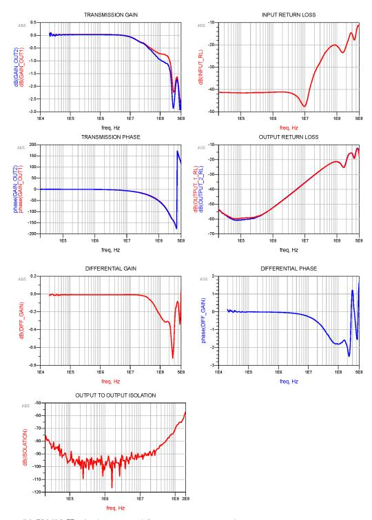
Figure 56: J2161A Typical measured frequency response data.
