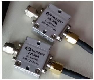
Figure 23: The P2130A DC blocker has a frequency response of 500Hz – 8GHz.
