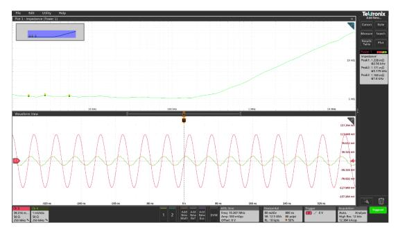
Figure 52: 2-Port Shunt-Thru Impedance measurement of a 1m Ohm (1.17m) resistor.
