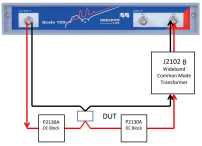
Figure 34: Connection diagram showing the placement of the J2102B common mode transformer. Inclusion of the transformer eliminates the low frequency distortion caused by instrumentation ground loops. P2130A DC blocks are only necessary when voltages greater than the Bode 100 VNA input voltage derated limits are exceeded.
