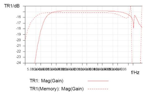
Figure 9: Frequency Response for the J2100A and J2101A injection transformer.
