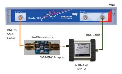
Figure 42: Measuring a low value resistor. The J2102A has been replaced by the J2102B.
