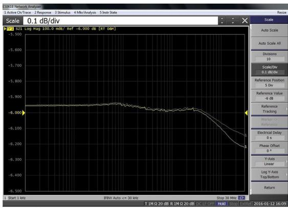
Figure 61: The 6dB splitter is accurate to within 0.25dB across the full frequency range of the instrument.
