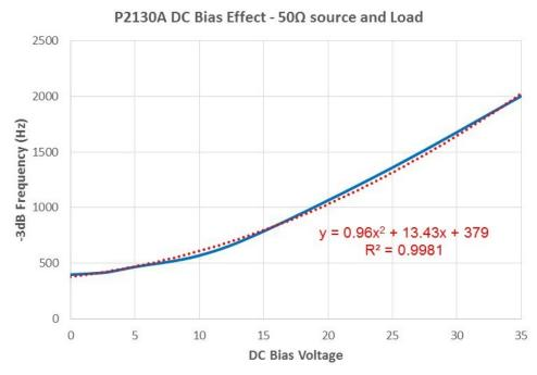
Figure 24: The effect of DC bias on the J2130A and P2130A frequency performance which shifts the - 3dB frequency.
