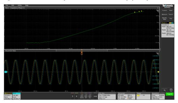
Figure 54: 2-Port Shunt-Thru Impedance measurement of a 3.3uH inductor.
