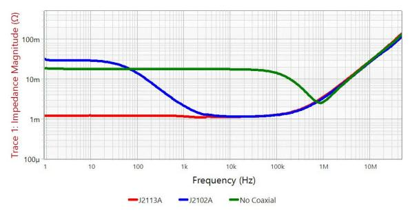
Figure 43: J2113A - J2102B - Comparison Plot. Measurement is of a 1mOhm resistor with the J2102B passive coaxial transformer, the J2113A Semi-Floating Differential Amplifier and with no ground loop breaker at all. The reduction in the error of the measurement is clearly seen.
