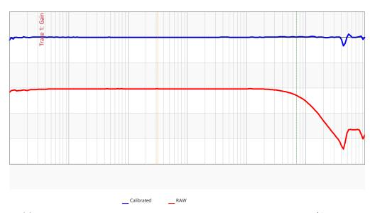
Figure 17: The current monitor transfer ratio measurement shows the 100mV/A (-20dB) transfer function from the modulation current to the current monitor output. Uncalibrated, the -3dB frequency is 700kHz. Calibrated the response is 10Hz-1MHz.
