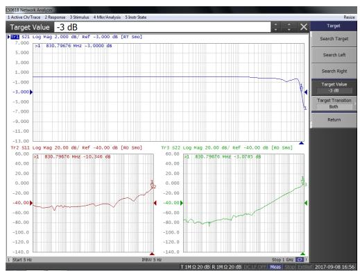
Figure 48: S21, S11, and S22 plots show 3dB S21 -3dB bandwidth @ 830MHz and S22 -6dB bandwidth @ 635 MHz.
