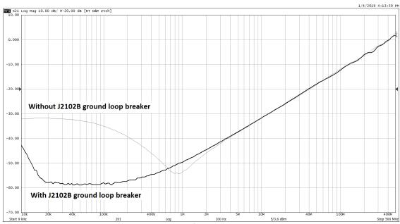
Figure 37: Impedance measurement of a  $1m\Omega$  resistor with and without the J2102B common mode transformer using the Copper Mountain S5065 VNA.
