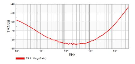
Figure 36: Common Mode Frequency response of the J2102B.
