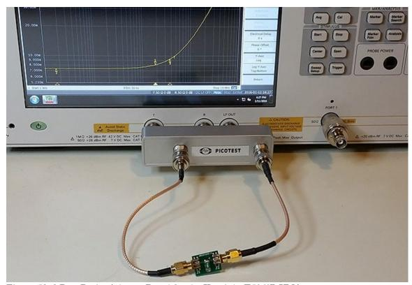
Figure 58: 2 Port Probe Adapter Panel for the Keysight E5061B VNA.
