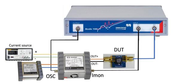
Figure 5: Sample setup for the Line Injector (J2121A) used to measure an inductor under DC bias conditions.
