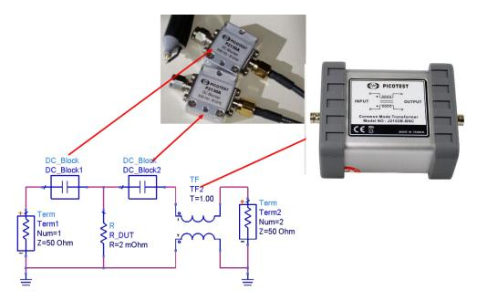
Figure 35: Electrical connection diagram showing the placement of the J2102B and P2130A DC blockers for a 2 port shunt impedance measurement.
