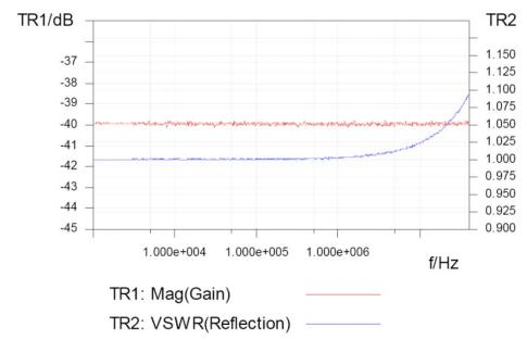
Figure 29: 40dB attenuator frequency response.
