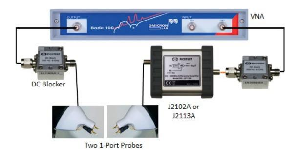
Figure 45: Test setup for measuring the in-circuit output impedance using two 1-Port PDN Probes (P2100A). The J2102A has been replaced by the J2102B.
