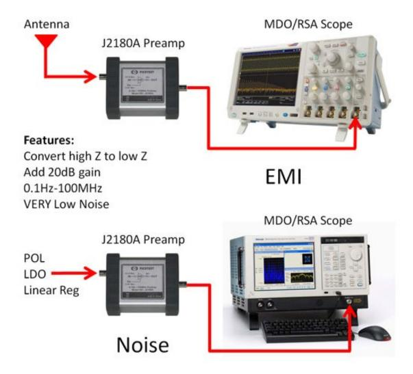
Figure 31: Sample setups for the J2180A Preamp used for noise and EMI measurements.
