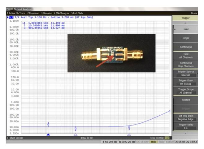
Figure 60: 10 milli-ohm Resistor measurement using the Keysight E5061B VNA GP Ports and the Picotest J2160 adapter.
