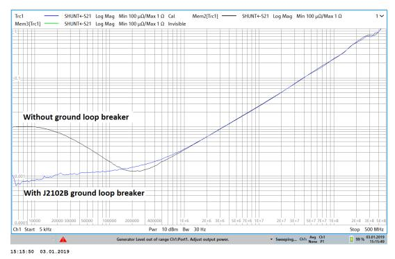
Figure 38: Impedance measurement of a  $1m\Omega$  resistor with and without the J2102B common mode transformer using the Rohde & Schwarz ZNL VNA.
