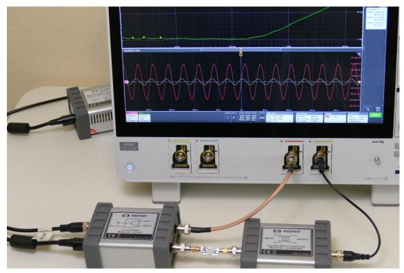
Figure 51: – Tektronix Series 6 test setup to perform the 2-port shunt-through impedance measurement using the Picotest J2161A active splitter (left) and the J2102B common mode transformer (right).
