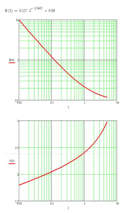
Figure 19: the voltage drop of the J2123A is graphically represented above.
