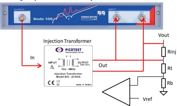
Figure 8: Injection Transformer Connections for stability measurements.
