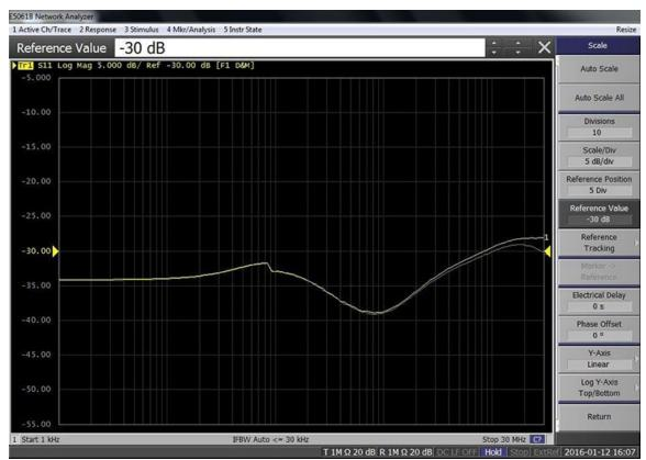
Figure 64: The return loss of the 6dB splitter legs is better than 25dB over the full measurement range of the instrument.
