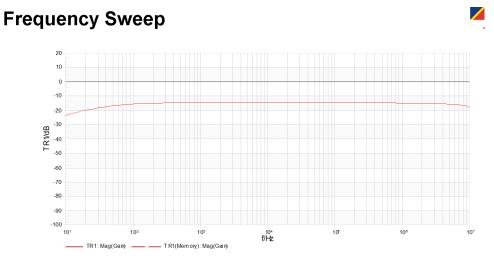
Figure 10: Frequency Response for J2101A injection transformer.
