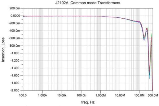
Figure 40: J2102A Insertion Loss Graph.
