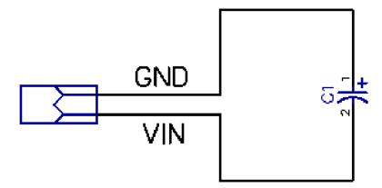
Figure 21: Internal input capacitor polarity.
