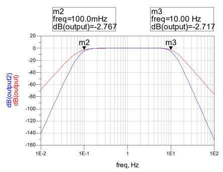
Figure 33: Frequency response of a single filter (red trace) and 2 cascaded filters (blue trace).
