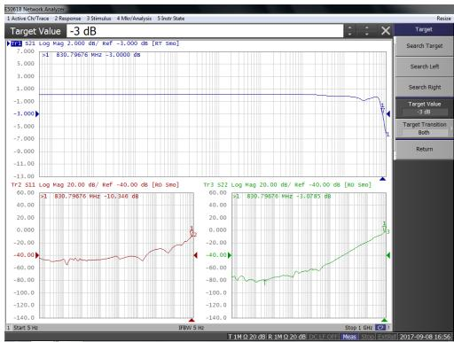
Figure 55: S21, S11, and S22 plots show 3dB S21 -3dB bandwidth @ 830MHz and S22 -6dB bandwidth @ 635 MHz.
