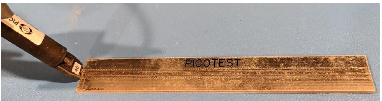
Fig. 9 - TDR Setup on 50Ω Microstrip Transmission Line with the P2105A Probe.
