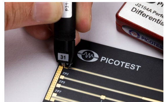
The Picotest P2105A browser probes have a usable bandwidth greater than 15GHz.
