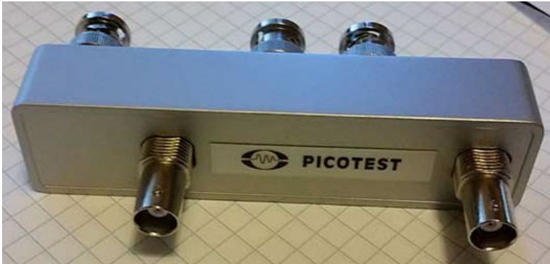
Figures 4: Picotest J2160A 2-Port Probe Adapter Panel that converts the low frequency E5061B T/R port into a 2-port shunt through configuration.
