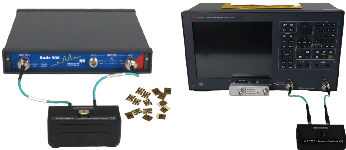
Figures 3: The CTF is connected to the Bode 100 (left) and the Keysight E5061B (right) on the S-parameter ports. You can connect to the low frequency T/R ports via the Picotest J2160A 2-Port Probe Adapter Panel.
