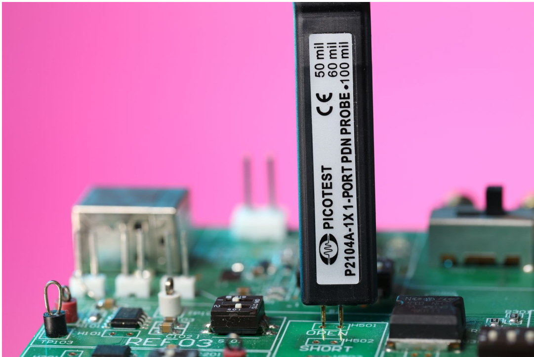
Figure 23: The center pin is the positive pin on the P2104A 1-port probe.
