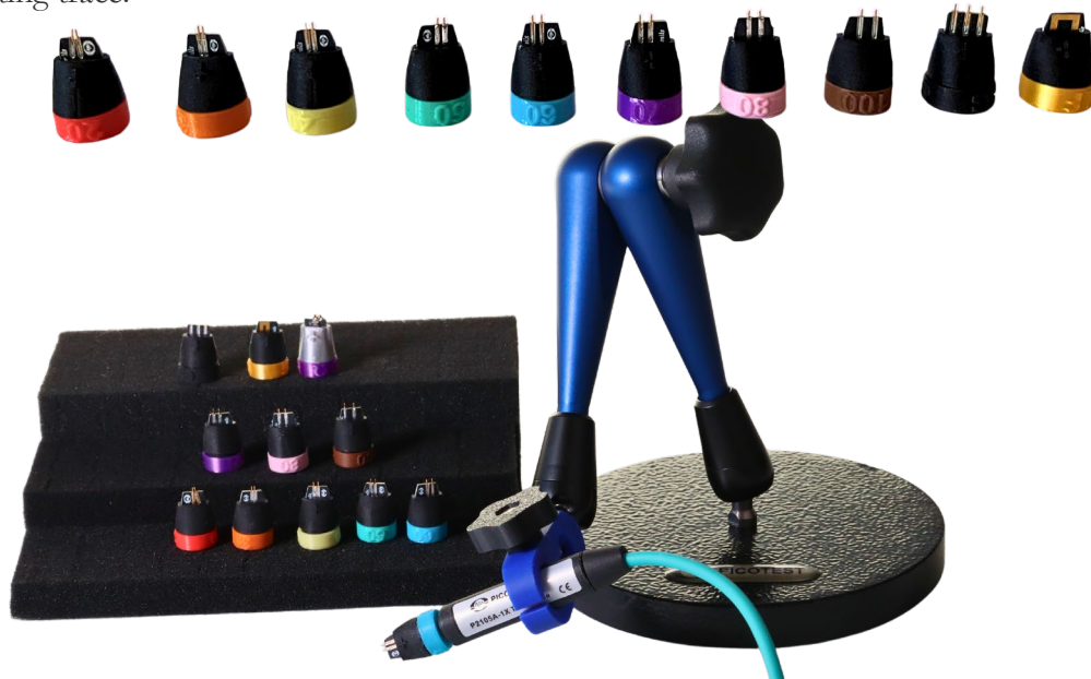
Figure 7: The P2105A 5 in 1 probe uses interchangeable heads to change functionality. Probe heads are available for TDR/Ripple/Impedance, transient load current stepping, and near-field measurements. Different probe pitches are also color-coded.
