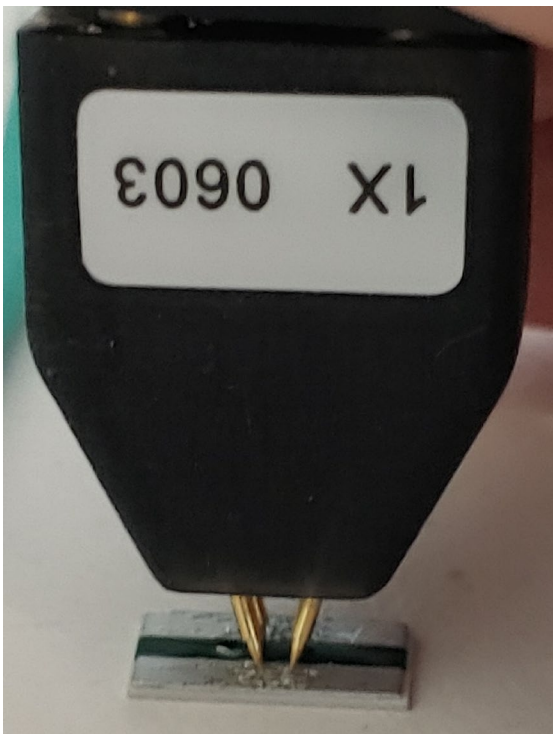
Figure 20: A 2-port measurement using the P2102A probe. Pressure is needed to seat the four pins firmly in place. The probe head should match or be larger than the capacitor being measured across. Two pins go on each side of the capacitor.
