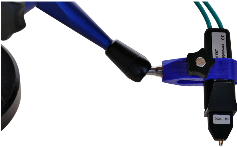
Figure 21: Two signal lines go on the positive side of the capacitor and two ground lines go on the ground side of the capacitor. The positive probe side is the side with the label.
