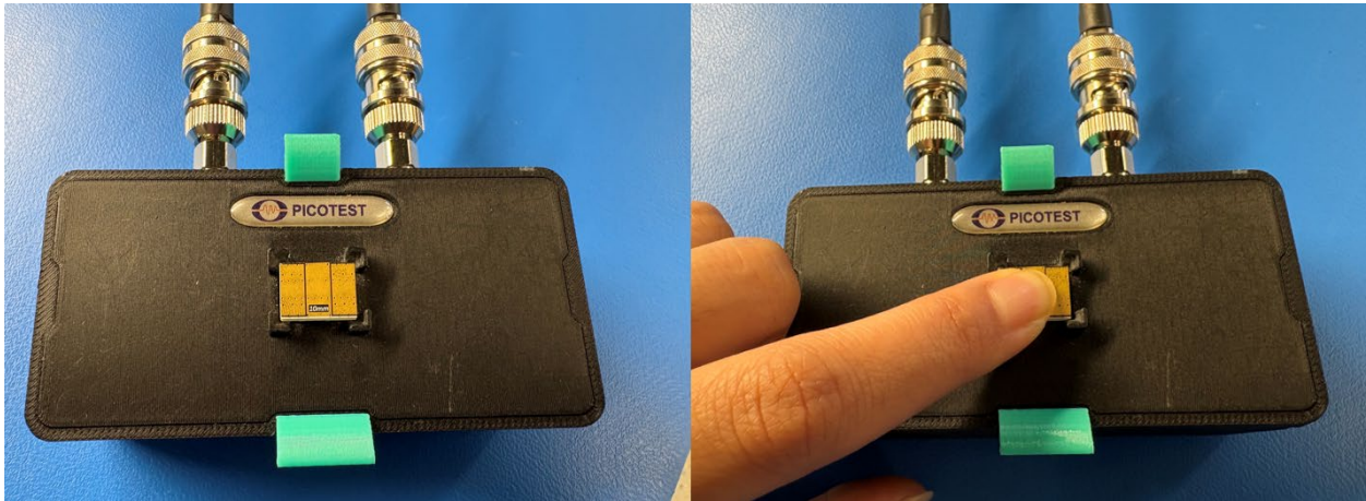
Figure 3: With the Calibration Board on the CTF, Press Firmly and Hold for the Entire Duration of Calibration Step
