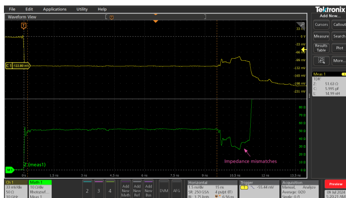
The TDR analysis provides an impedance waveform for the trace in the above figure. The impedance, capacitance and inductance of the waveform across marked regions are displayed in a measurement badge. The lower impedance in the center of the screen corresponds to the wider section of the PCB trace.
